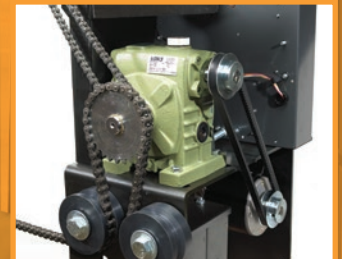
Full Size Gearbox heavy-duty 30:1 ratio gearbox
